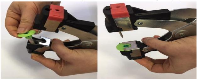
• It is vital to insert the female part of the tag first as the tag will not fit correctly otherwise. Make sure it is secure and held in place by the clamp.
